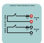
MSS-2##C-004: Series 1k resistor on Circuit A and on Circuit B. One instance shown at right:
